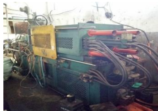
Gambar 2. Mesin injection moulding KT 105 G
