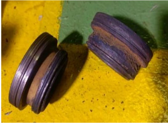
Gambar 3. Seating exhaust valve cylinder nomor 1 generator nomor 1
