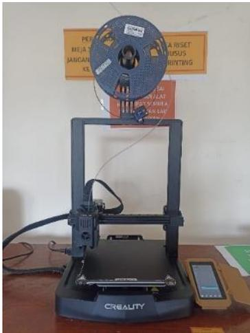
**Gambar 7.** Mesin Printer 3D Creality Ender 3 V3 KE
