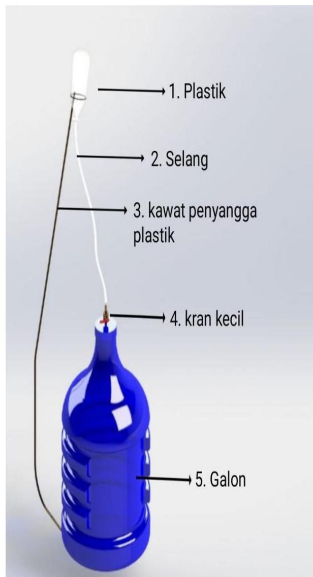
**Gambar 2.** Digester tipe *batch*
